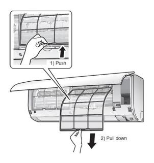
If the filters don't clean easily, wash the air filters with neutral detergent thinned with lukewarm water, then dry them in the shade.
