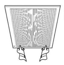
Ensure you support the grille face while undoing the screws / clips to avoid it freely swinging downwards.
