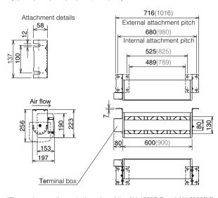
\*Figures in parentheses is the value of the AH-1509S-E and AH-2009S-E. Unit (mm)
